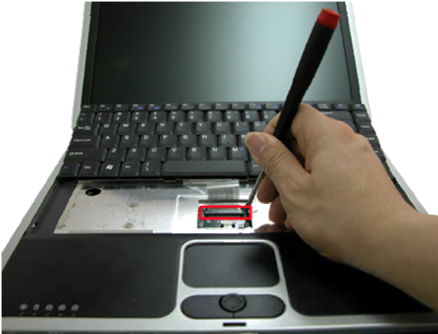
Fig. 16 Disconnect keyboard flat cable
